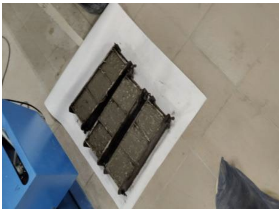
Fig.4– Hybrid Basalt Fiber Reinforced concrete casted prior to testing
