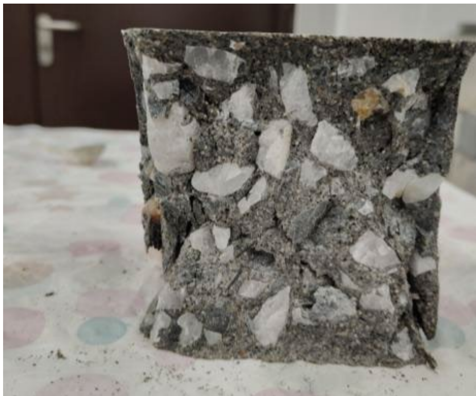
Fig.6– Hybrid Basalt Fiber Reinforced Concrete Cube after failure
