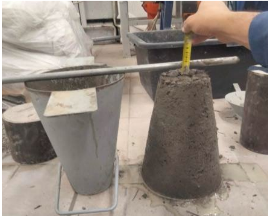
Fig.3– Workability test on a Hybrid Basalt Fiber concrete
